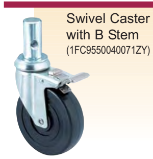
Type B Stem 1.25" x 2-1/2" round stem w/7/16" hole located 1" up
