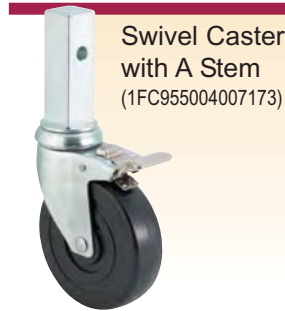
Type A Stem 1.25" x 4" square stem w/7/16" hole located 2-1/2" up
